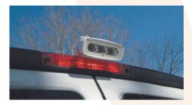
Provides additional lighting & security when loading and unloading prisoners
