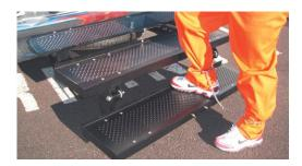
**REAR FLIP DOWN STEP**Attaches to rear step for safer entry & exit of the van (May interfere with reverse proximity sensors).
