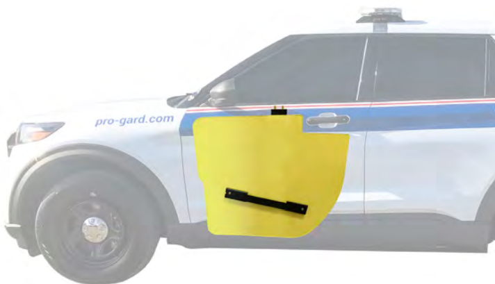
Ballistic Door Panels illustrated on the 2020 Ford Police Interceptor Utility
