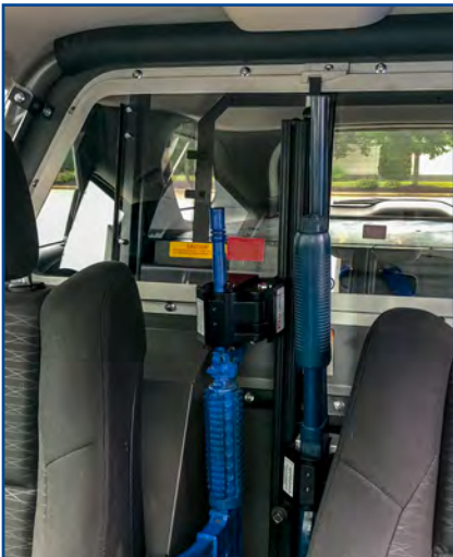
The Tri-Lock Vertical Partition Mount shown in the 2018 Dodge Durango
