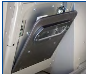
Shield deployed upon releasing T-handle
