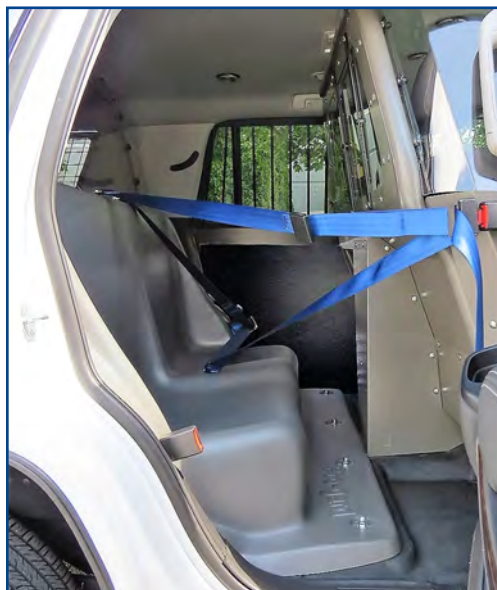
Transport Seat with optional Outboard Seat Belts shown in the 2018 Chevy Tahoe
