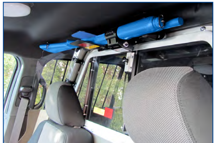
The G5000 Series Gun Rack shown in the 2013-2019 Ford Police Interceptor Utility
