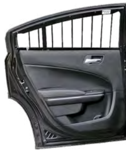
Steel Bars with OEM Door Panel
