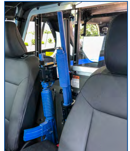
The Tri-Lock Vertical Partition Mount Gun Rack shown in the 2020 Ford Police Interceptor Utility
