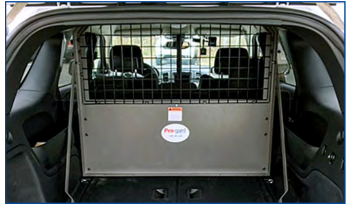
Wire Screen Cargo Barrier shown in the Dodge Durango
